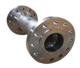
Flanged assembly consisting of a series of orifice plates to produce a specified reduction in line pressure or to create a critical flow, giving controlled flow rate regardless of changes in downstream conditions. In-house expertise covers all aspects of design and manufacture associated with restriction of pressure for control purposes.
